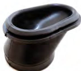
Ref. 015004 • s10-10607 GOMA FILTRO/ CARBURADOR AIR BOX/CARBURADOR RUBBER Scorpa T Ride 250 F
